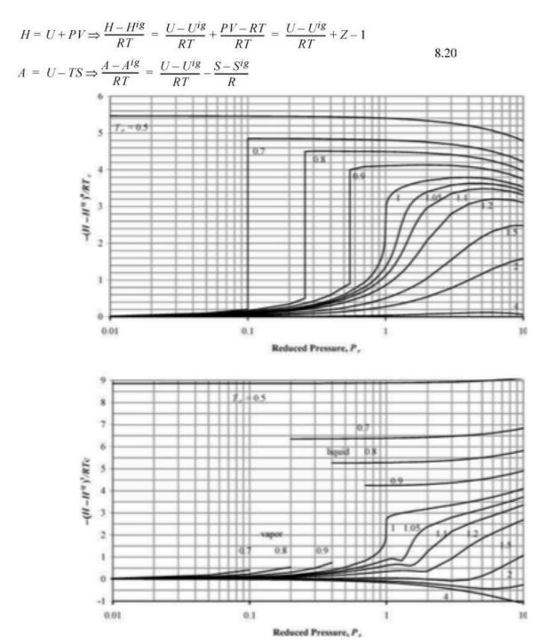
Figure 8.7. Generalized charts for estimating  $(H-H^{ig})/RT_c$  using the Lee-Kesler equation of state.  $(H-H^{ig})^0/RT_c$  uses  $\omega=0.0$ , and  $(H-H^{ig})^1/RT_c$  is the correction factor for a hypothetical compound with  $\omega=1.0$ . Divide by reduced temperature to obtain the enthalpy departure function.
